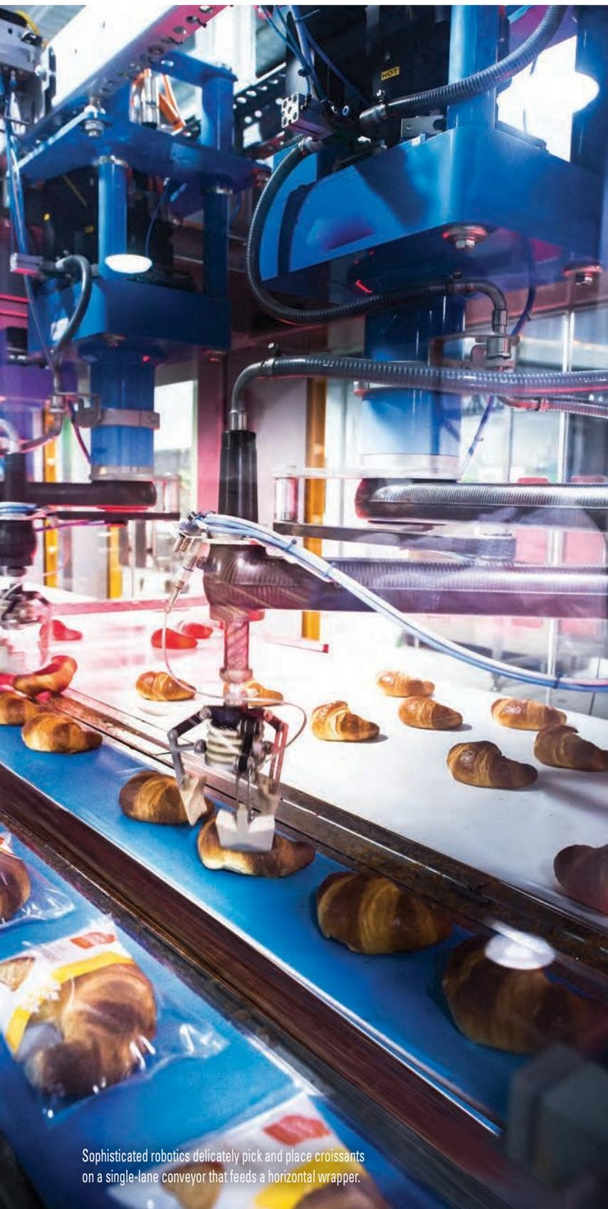
Sophisticated robotics delicately pick and place croissants on a single-lane conveyor that feeds a horizontal wrapper.
